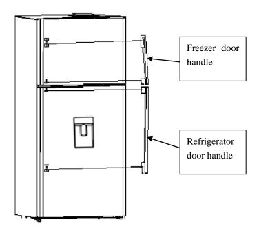
Separately set the two end covers handle in the handle seats of the freezer door, then press the door handle on the door and push down with too much force. Then gently support upwards with hands to check the handle whether fall off or not. Installing the refrigerator door handle is using the same methods.
